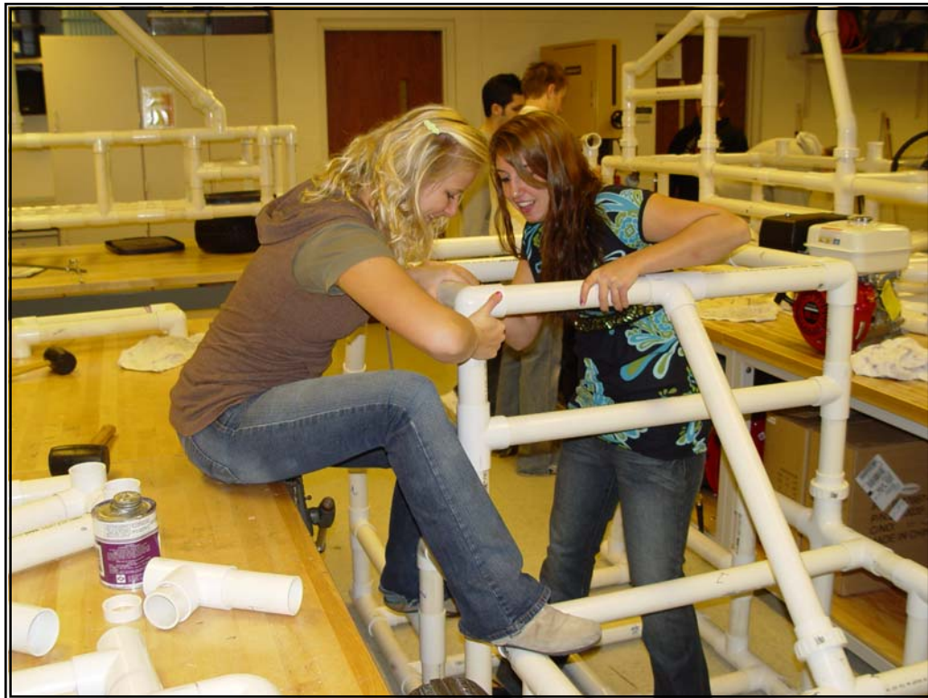
(Top: Making room for the torque convertor, Bottom: Megan Felcyn and Sarah Mozdrzech displaying teamwork gluing together the rollcage)
