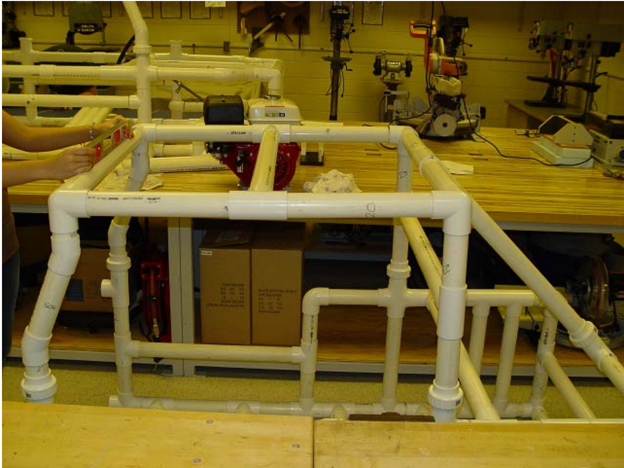
Roll cage isn't quite level because we glued things in the wrong order
