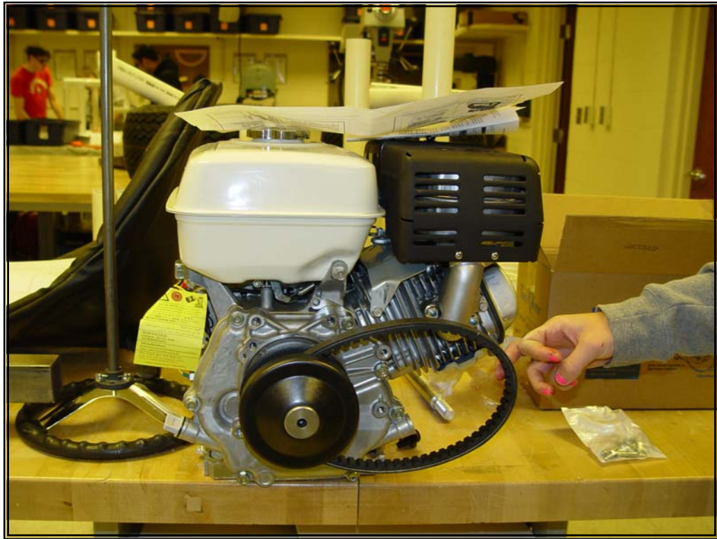
(Top: Assembly of engine with the modified torque convertor. Bottom: Eric Murphy gluing the PVC)
