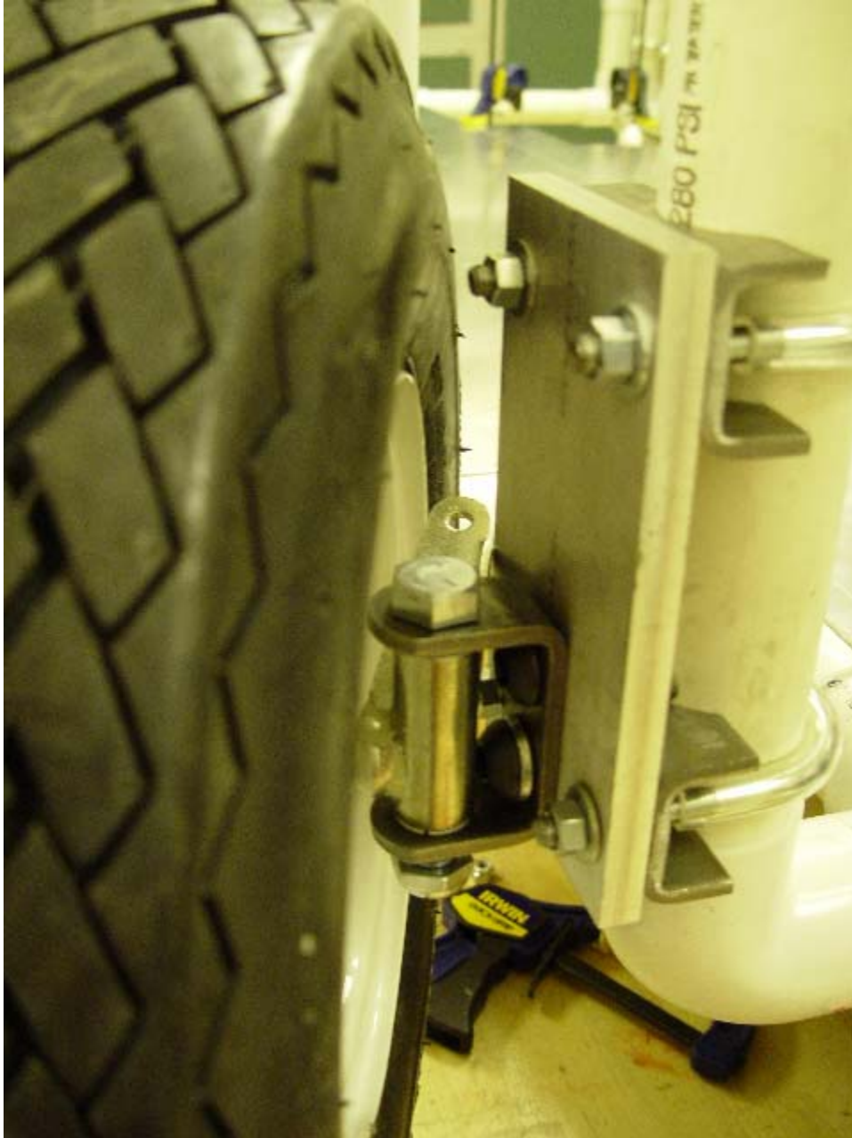
Front steering plate was too large and U-bolt rubbed against tire
