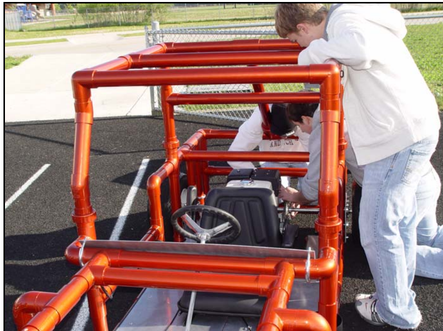
Figure 1 Fixing the chain after it popped off.
