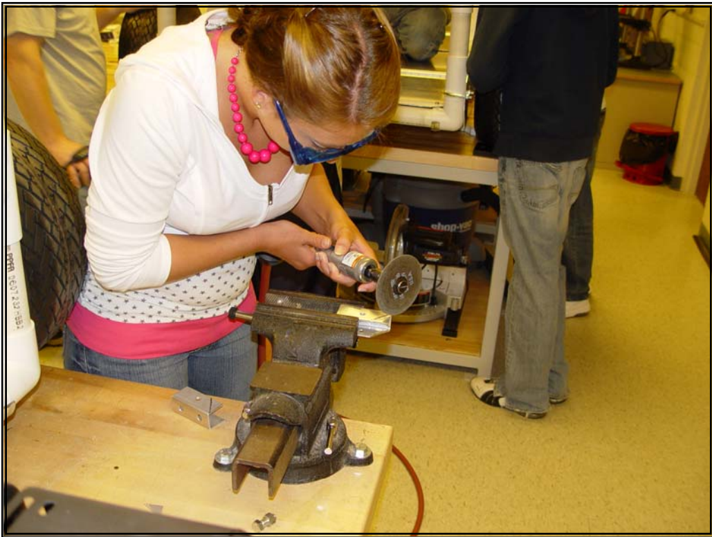
(Top: Mock up of rear axle, Bottom: Sarah Mozdzech grinding the pedal brackets)
