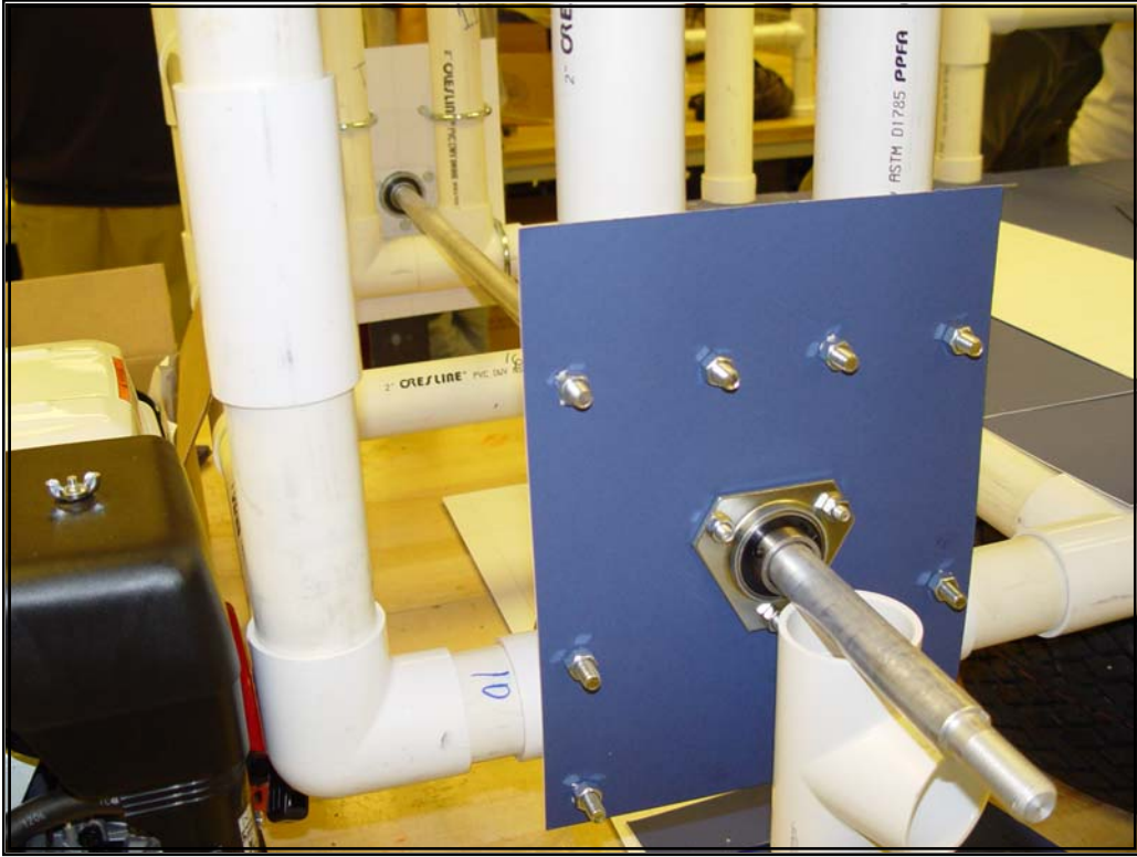
(Top: Mock up of rear axle, Bottom: Sarah Mozdzech grinding the pedal brackets)
