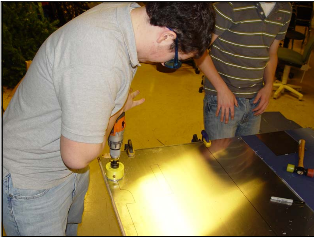
(Top: Aluminum floor completed, Bottom: Ryan Stevens cutting the floor plate)
