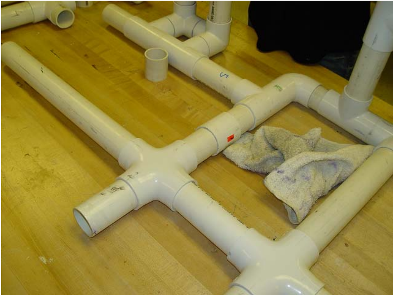
Fixing front-end problem with couplers
