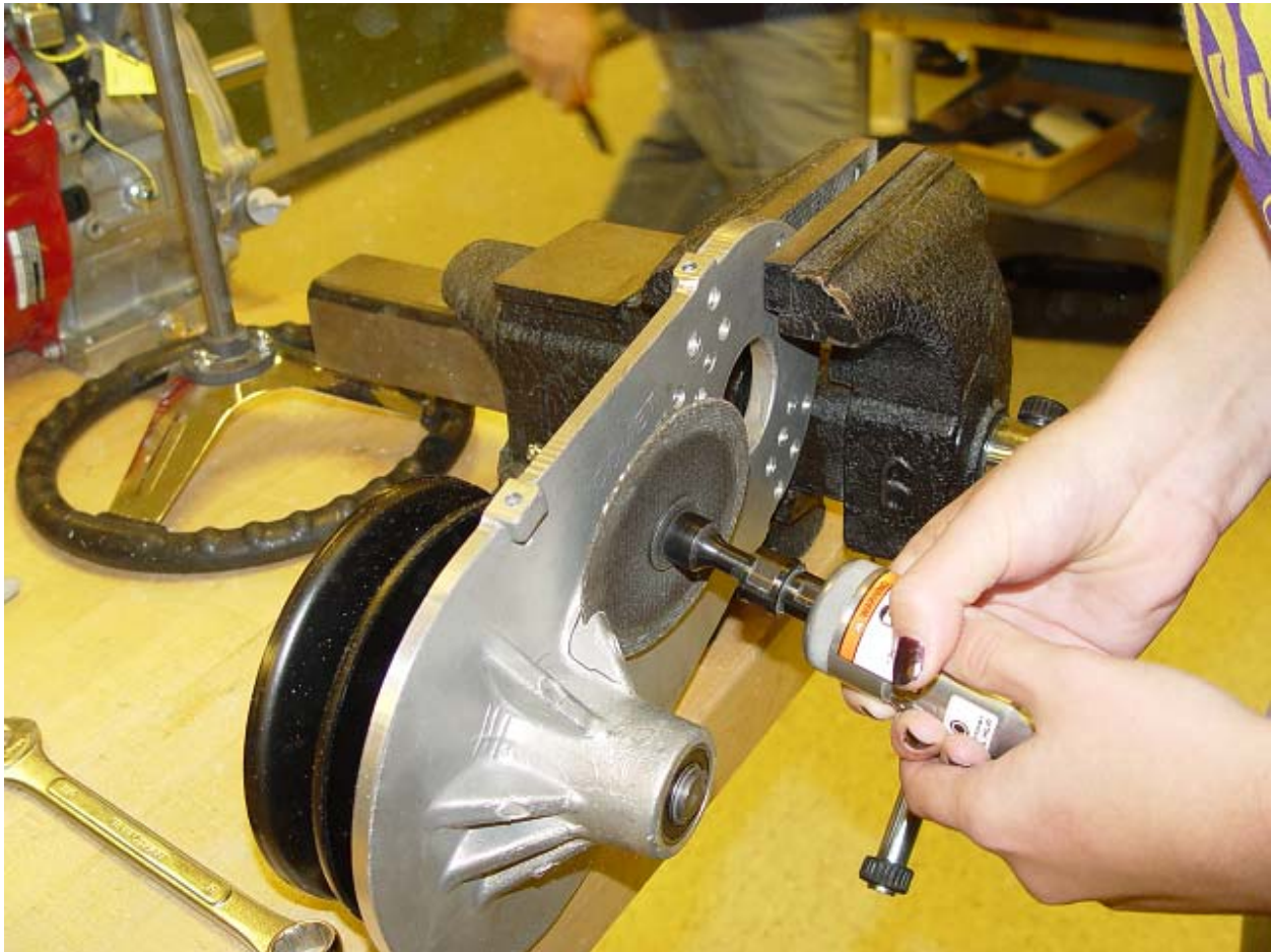
Cutting torque-converter support so it will fit on engine
