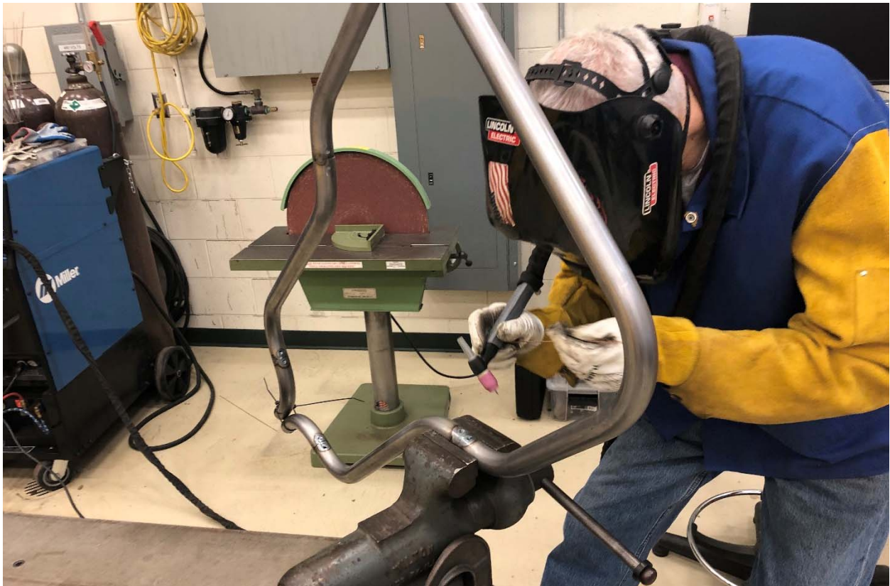
The welding of the main frame (shout out to Mr.D)
