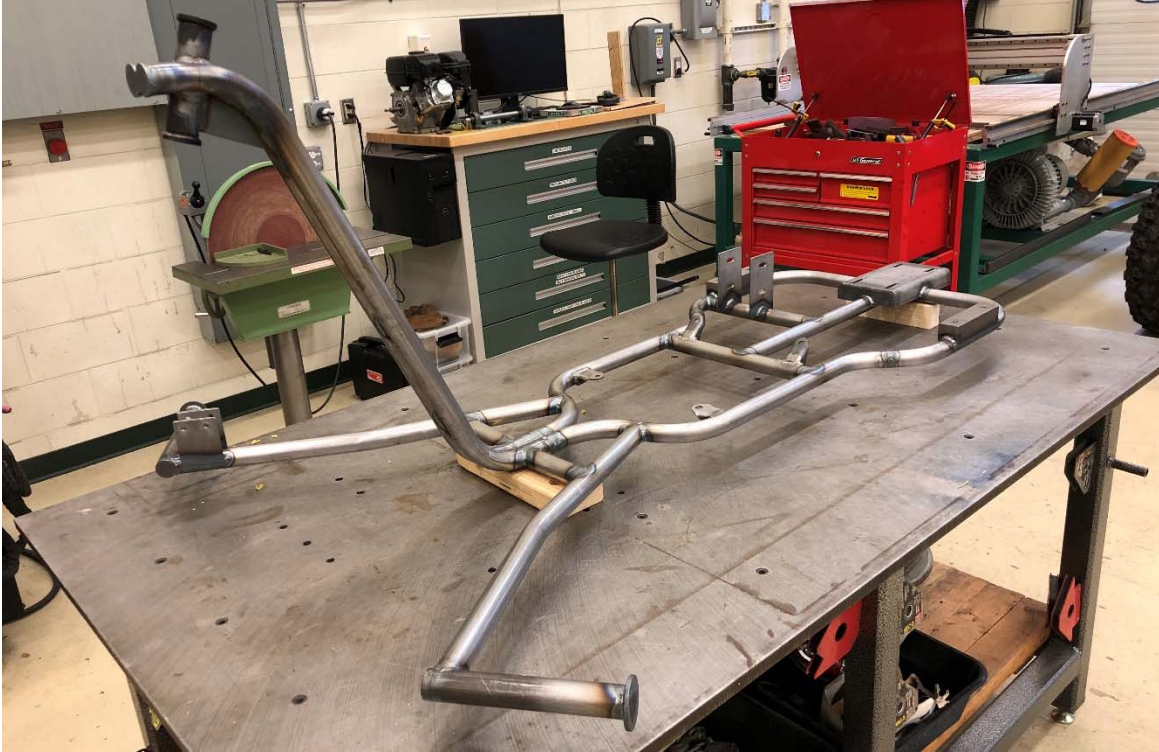
Completely welded up frame, just needs sanding.
