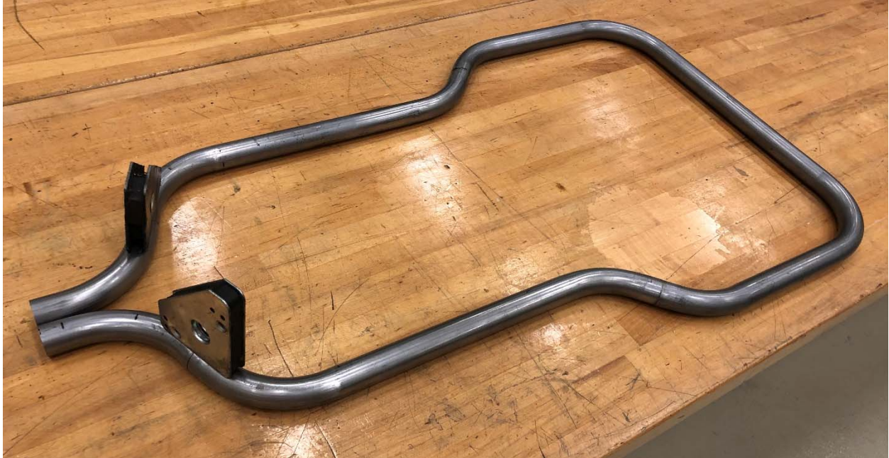
Main frame bent and cut, just needs to be welded up.
