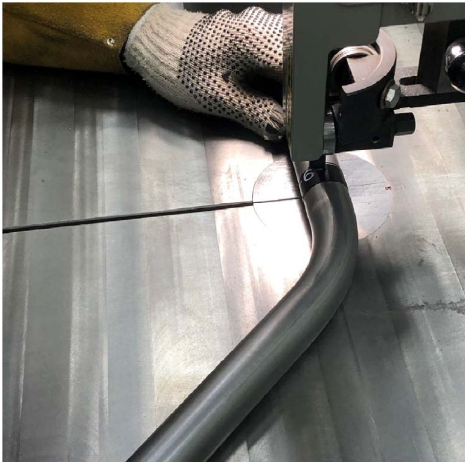
After the tubes were all bent, they needed to be cut down to the proper length.
