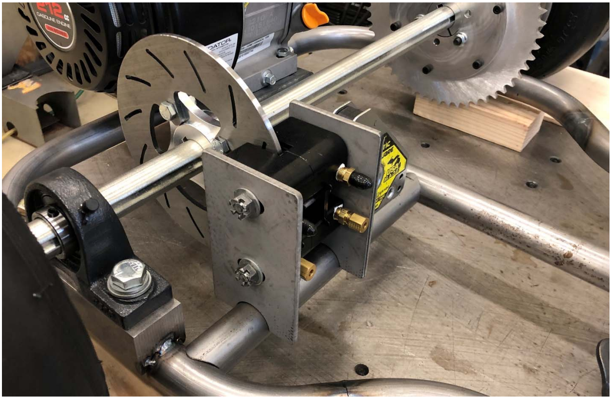
Rear brake caliper and engine mount to be welded in.
