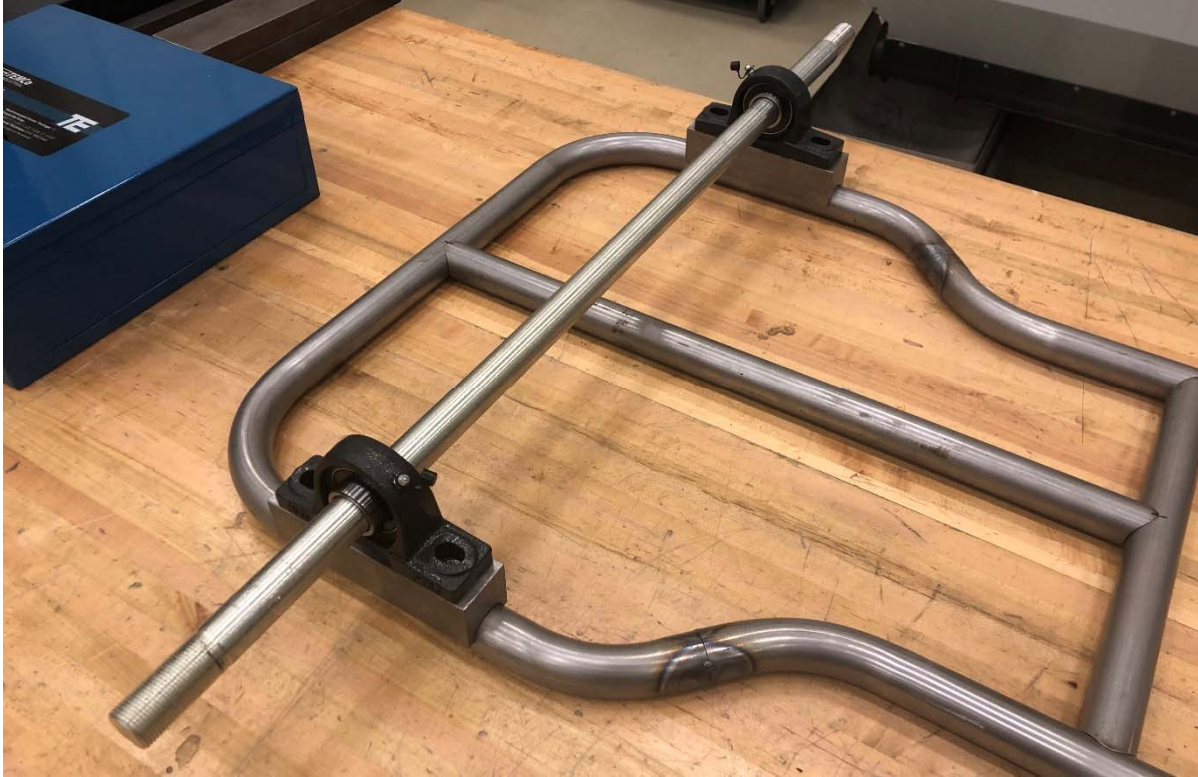
Pillow block bearing mounts and support tubes in place ready for welding.
