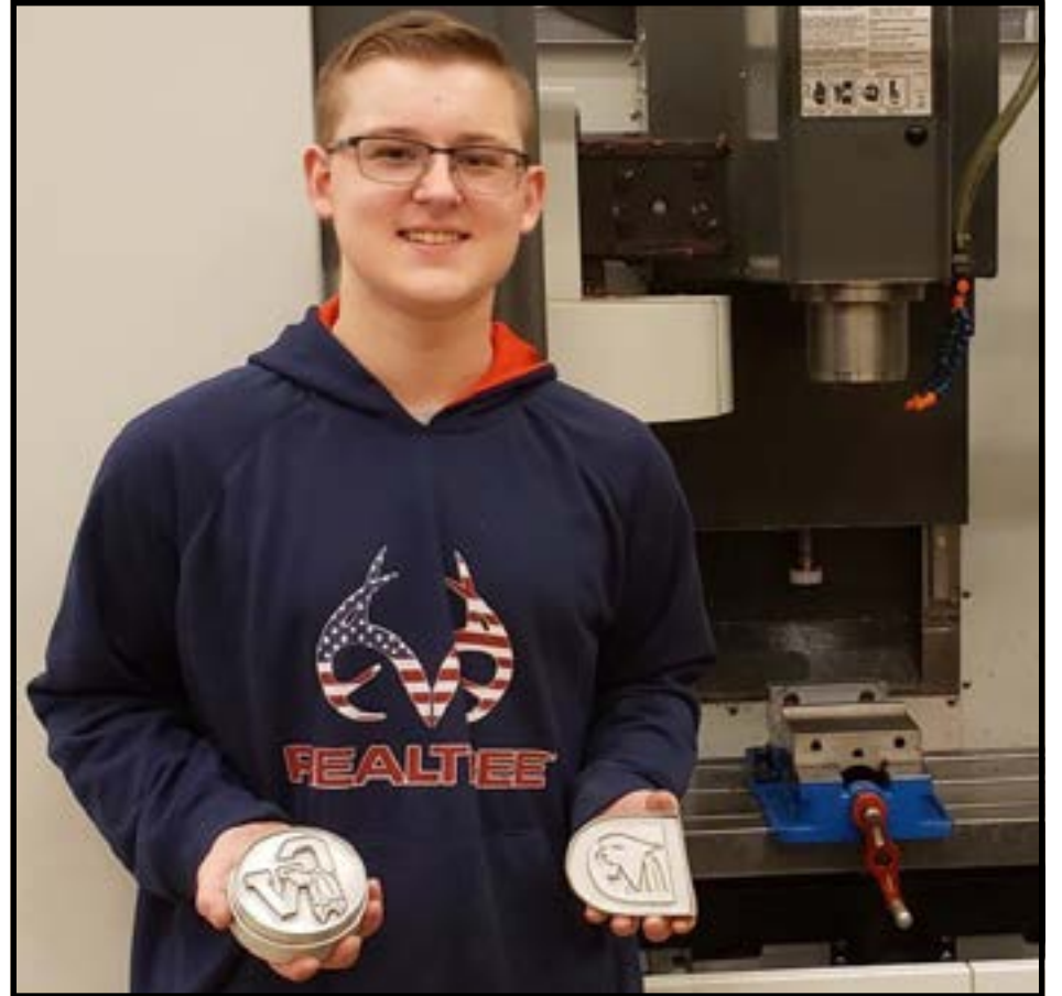
Work-based learning and community service come together in this project: CTE Design Technology Senior Noah Zielinski is holding the custom-made cookie molds that he fabricated for the CTE Culinary Arts program. The process started with designing the molds using AutoCAD software; converting the 2-D CAD drawings to 3-D models with Inventor software; creating wood prototypes using Mastercam software; involved several iterations and tweaking; and culminated in metal fabrication using a Haas CNC mill. Culinary Arts students can now make delicious cookies with the Chippewa Valley and Dakota High Schools' logos imprinted in them.
