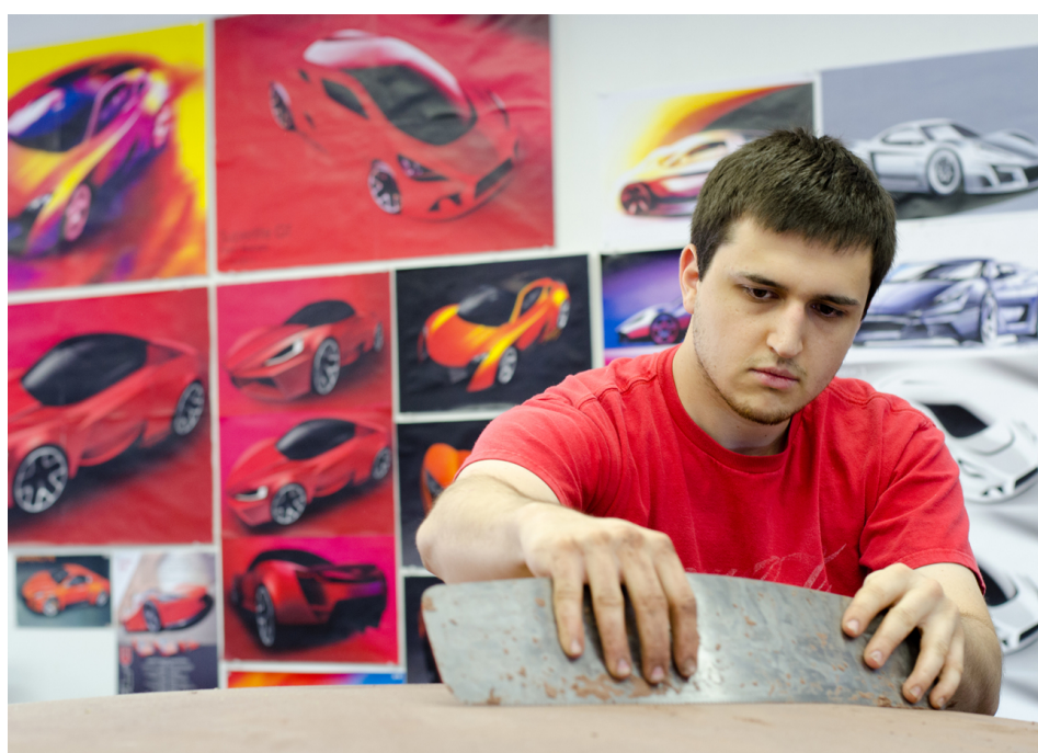
Dakota High School graduate Florin Blebea, shown here as he skillfully contributes to creating a full size, clay model of the Superlite Apex vehicle being manufactured by Superlite Cars LLC in Clinton Township.
